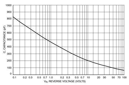
Figure 7. Typical Capacitance (Per Leg)
