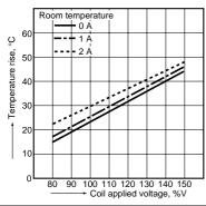
6.-(2) Coil temperature rise Tested sample: TK1-12V, 6 pcs. Measured portion: Inside the coil Ambient temperature: 70°C 158°F
