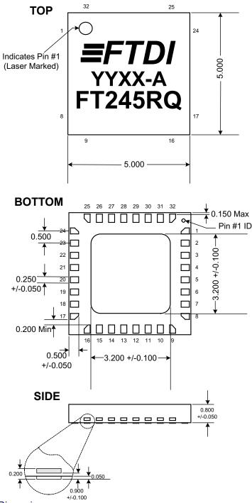
Figure 9 - QFN-32 Package Dimensions
