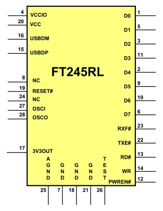
Figure 3 - 28 Pin SSOP Package Pin Out (Schematic Symbol)
