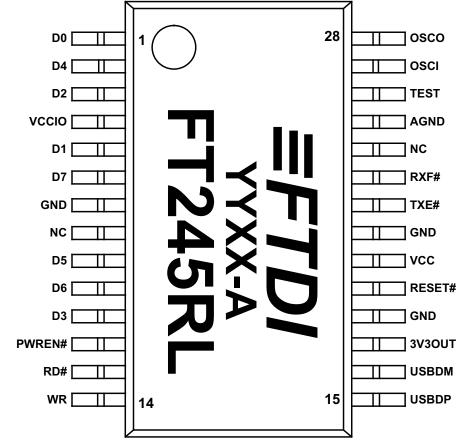
Figure 2 - 28 Pin SSOP Package Pin Out
