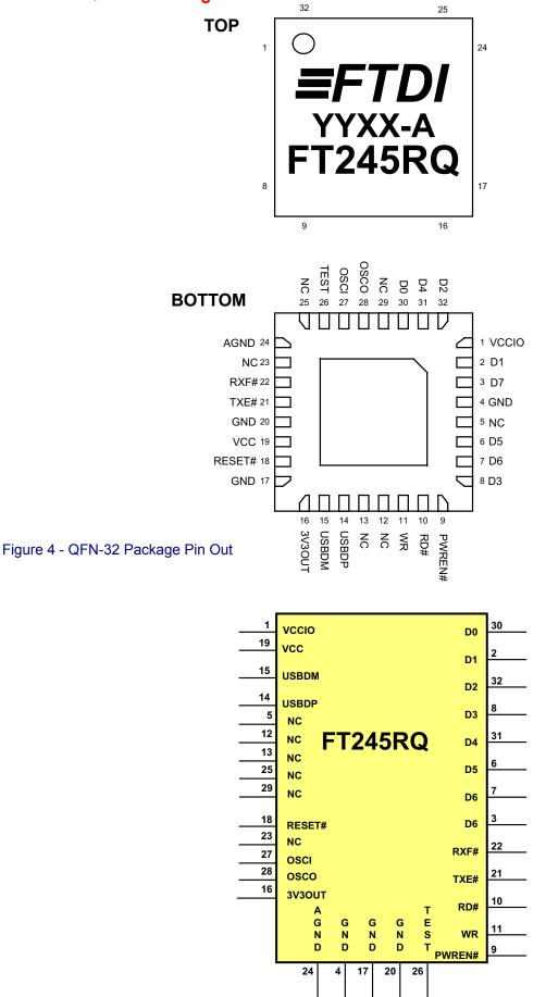
Figure 5 - QFN-32 Package Pin Out (Schematic Symbol)
