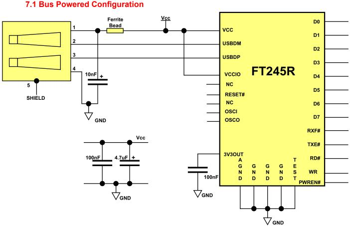
Figure 13 - Bus Powered Configuration
