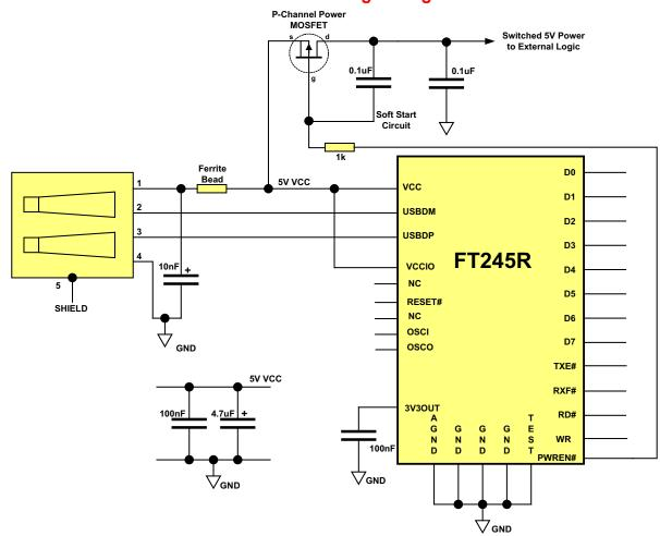
Figure 15 - Bus Powered with Power Switching Configuration
