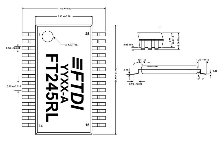
Figure 8 - SSOP-28 Package Dimensions
