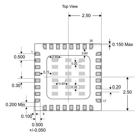
Figure 11 - Typical Solder Paste Diagram for QFN-32 Package
